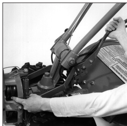
Figure 4-12: High range to low range. Shows moving belt from top-front pulley groove onto top-rear pulley groove.
